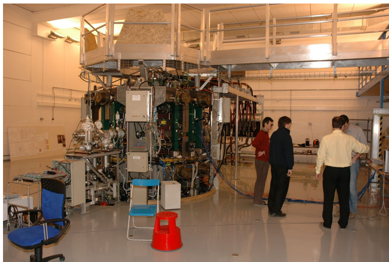
Figure 2.2: COMPASS before the first plasma, 9.12.2008. The Upper Link Board, gallery over the tokamak, vacuum systems and basic diagnostics including fast visible camera installed.
