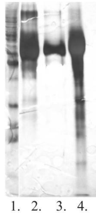
Figure 2. SDS-PAGE in 12% polyacrylamide gel detected by silver: 1. standard; 2. urine proteins before albumin extraction; 3. supernatant containing albumin after centrifugation; 4. urine proteins after albumin extraction.
