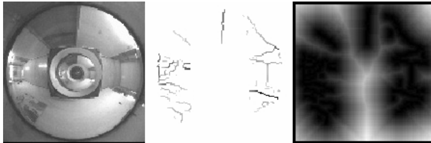
Figure 2.8: Important edges in an omni-directional image and the respective distance transform, reprinted from [17]
