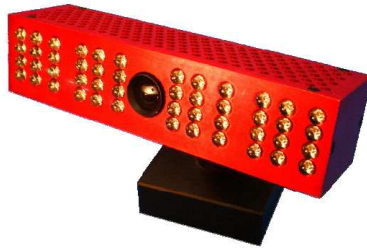
Figure 2.3: The time-of-flight Swiss Ranger sensor that is able to provide real-time depth maps of the environment, reprinted from [49]
