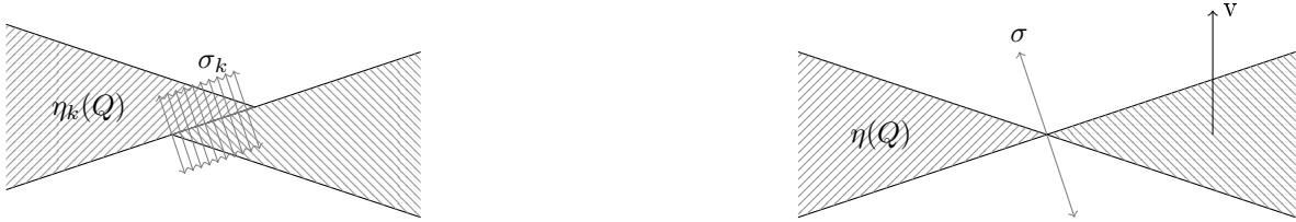
FIGURE 3. Approximate configurations and construction of a contact force without a fixed sign for all potential movement directions, as described in Remark 5.6. Specifically, moving the right hand solid in direction v is part of T_\eta(\mathcal{E}) but not T_\eta^0(\mathcal{E}) .
