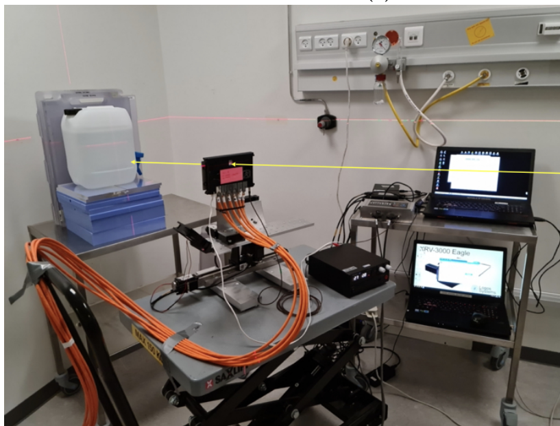
Experimental setup of the proton measurements. The device was irradiated with protons of different energy at the Danish Center for Particle Therapy. The proton beam direction is indicated.
