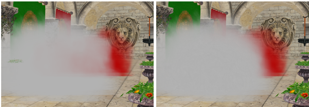
Figure 3.4 WBOIT gives much more weight on the smoke in foreground, yet, the result is still not perfect and overbleeding of vegetation can be spotted(left). Depth peeling (right)
