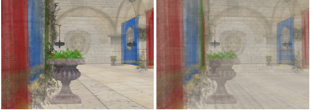
Figure 2.6 WBOIT (left) assigns more importance to closer surfaces in the Sponza scene with 25% transparency. Weighted average (right)
