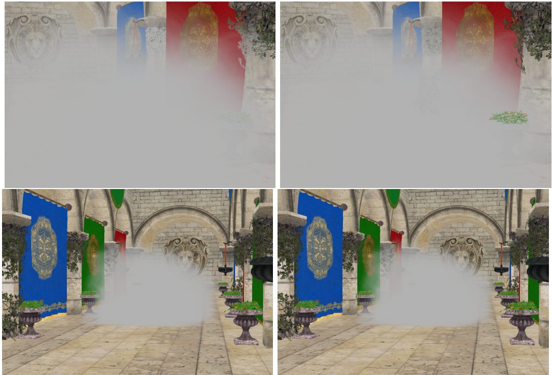
Figure 3.12 Adaptive Z improves the algorithm in the short distance without making it worse for further distances. Adaptive weight function w = 1/adapt(z)^5 \cdot \alpha on the left and a default weight function w = 1/z^5 \cdot \alpha on the right. Notice the overbleeding of vegetation on short distances with the default weight function
