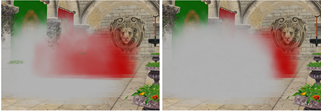
Figure 3.3 The color of the background red smoke is clearly visible even though it should be fully occluded by the gray smoke in foreground. This is a common case of overbleeding. Weighted average on left, depth peeling with 32 passes on right
