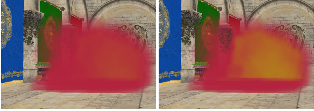
Figure 2.7 WBOIT with weight function w = 1/z^5 \cdot \alpha on the left. WBOIT with no weight function on the right. Notice the overbleeding of transparent vegetation and yellow smoke from behind the red one
