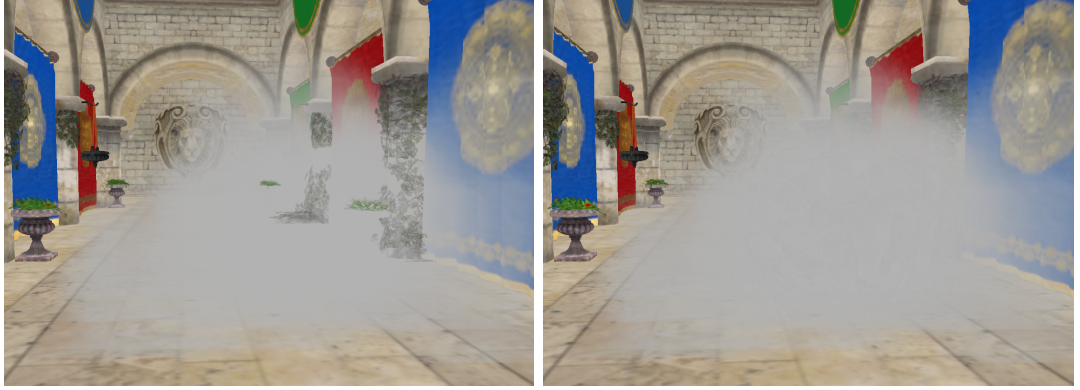
Figure 2.3 Overbleeding of transparent plants from behind the smoke particles in weighted average algorithm(left). Depth peeling (right)
