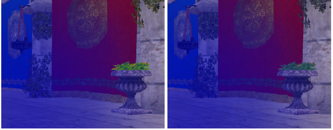
Figure 3.5 In the right side of the image, both the hanging vines and leaves in the pot are not properly occluded by the transparent blue smoke. This is due to them getting assigned a small importance from the used weight function ( W = 1/z^5 \cdot \alpha ) - WBOIT (left). Depth peeling (right).
