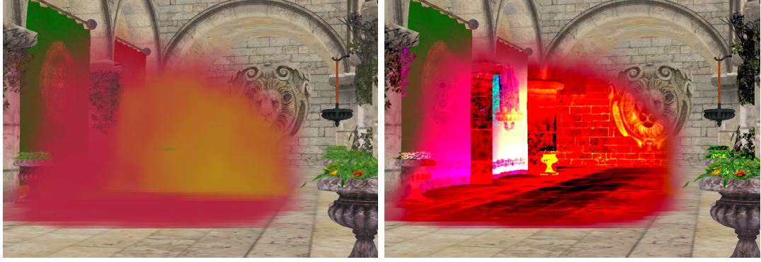
Figure 3.10 Overbleeding of vegetation and a yellow smoke from behind the red one in weighted average (left). Weighted sum overbleeds much more and reveals even the solid background.
