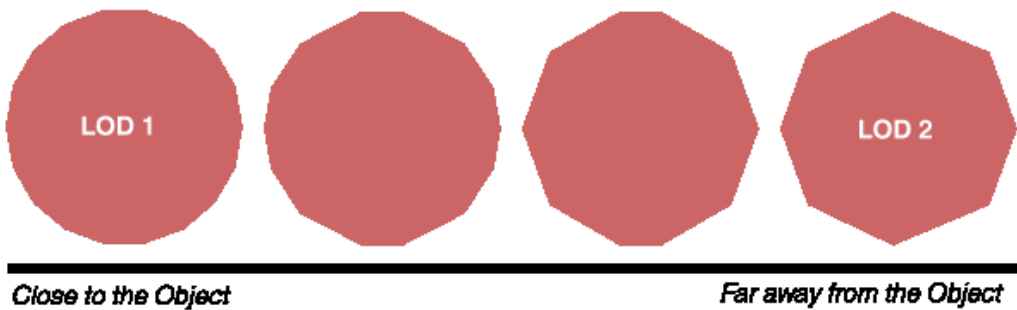
Figure 7 An illustration of geomorphing for transition between 2 levels of detail. Wikipedia - Popping (computer graphics). 3
