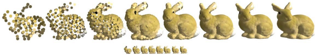
Figure 8 Model of Stanford Bunny consisting of varying amount of Blue Surfels. Note that the size of the surfels is not representative of actual rendering. Source: (Jähn, 2013)
