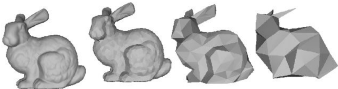
Figure 3 Comparison of different LoD levels on the Stanford bunny model. Source: YouTube! 1
