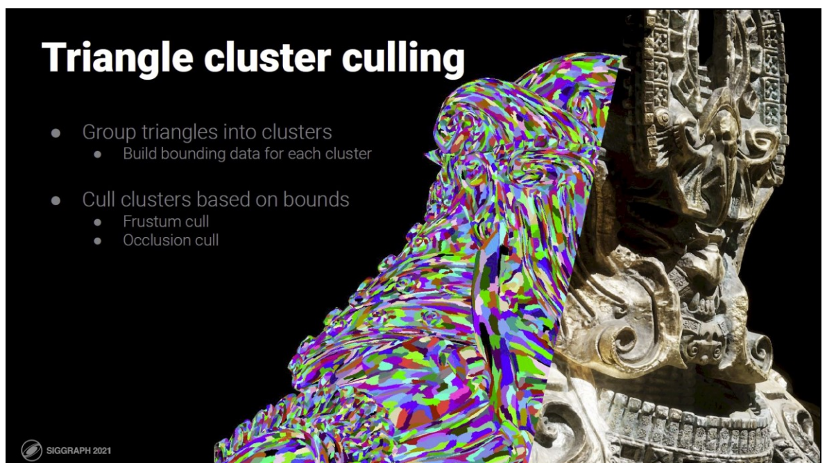
Figure 10 Nanite and its clustering of triangles. Source: Nanite – A Deep Dive presentation at SIGGRAPH 2021. 5
