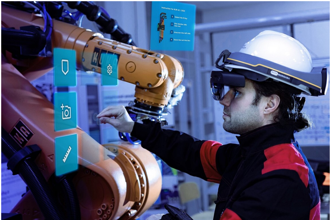
Figure 1 FMVoyager displaying additional information including maintenance steps, over the real environment. Courtesy of Pocket Virtuality
