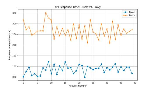
Figure 7.4: Response time of direct SAP Service Layer call in contrast of Proxy API
