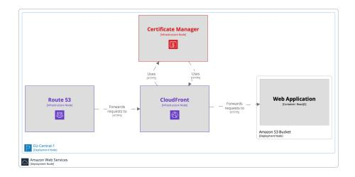
Figure 6.1: C4 Deployment diagram of static web application in AWS
