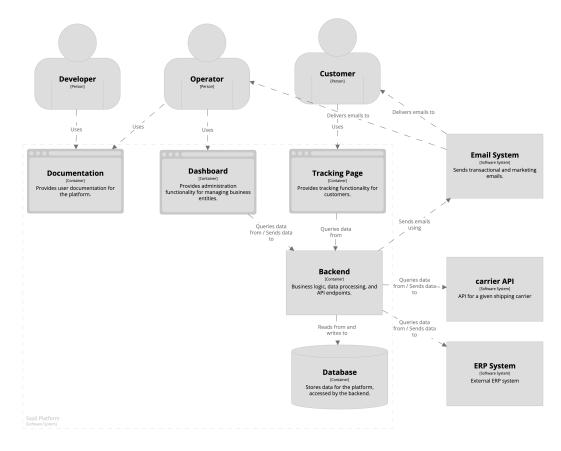
Figure 3.5: C4 container diagram of the software system
