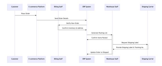
Figure 2.1: Sequence diagram of order dispatching process
