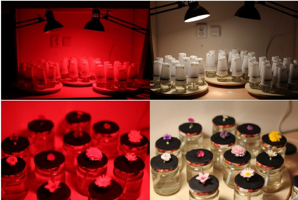
Fig. 3: Experimental room. Left: rating under red light, right: rating under normal yellow light. Top: situation during rating. All flowers are covered by numbered cups and placed on rotating plates. Participants only uncover and rate one flower at a time. Bottom: illustrative setting with all flowers uncovered. Flower colors are indistinguishable under red light.
