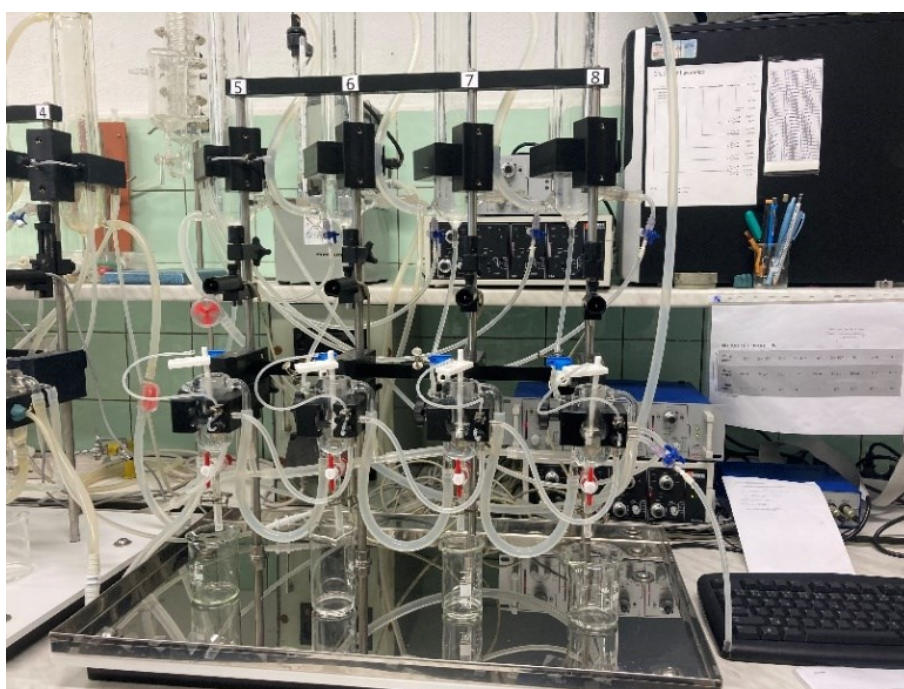
Obrázek 11 - Aparatura na izolovanou tkáň - Multi chamber tissue bath system
