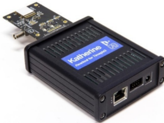
Figure 1.5: An image of the Katherine readout device [11]
