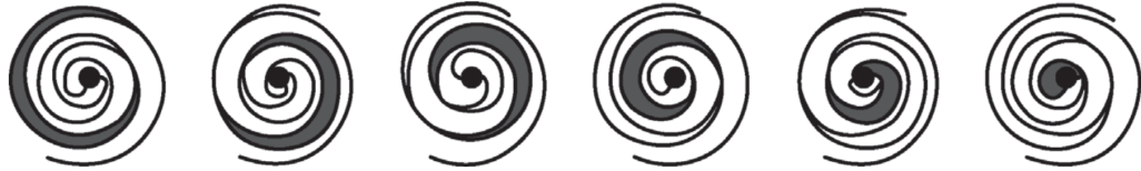
Figure 1.2: Gas path in scroll pump. Adapted from [3].
