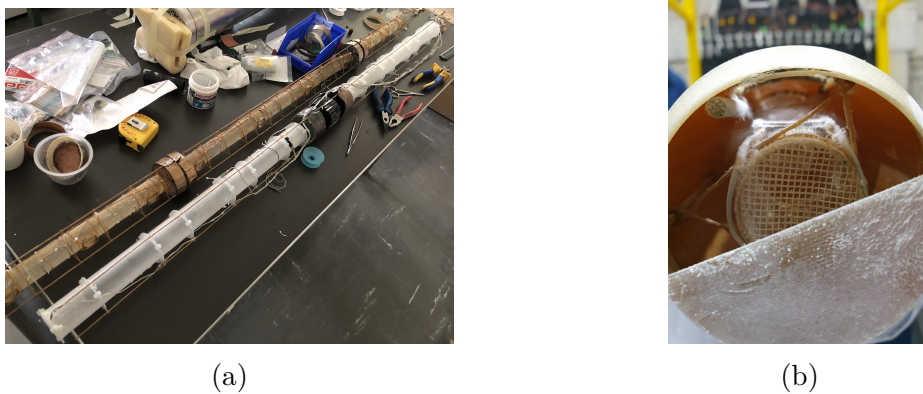
Figure 3.12: Photos of the polarised target holder, picture (a) shows the full target holder including the cables, and picture (b) shows the cross-section of the target holder with the ^3\text{He} pipe visible in the upper left part
