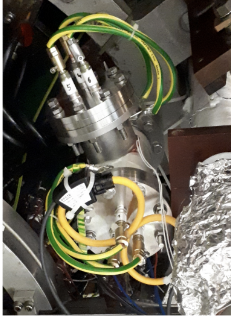
Figure 3.58: Connection of the special divertor tiles segments in grounded configuration.
