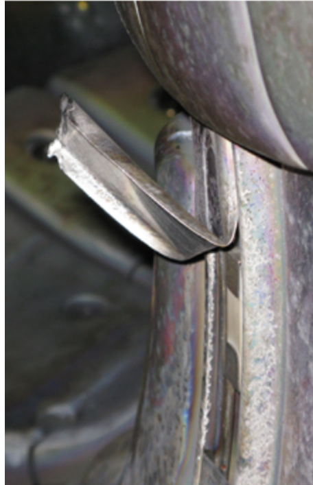
Figure 3.1: Magnetic coils casing damaged during a disruption.
