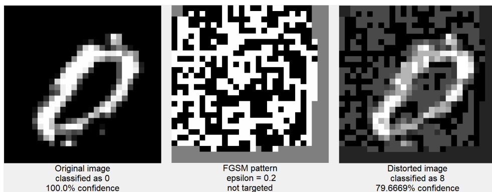
Figure 6.7: The original image was correctly classified as 0 with 100% confidence, while the adversarial example was classified as 8 with almost 80% confidence
