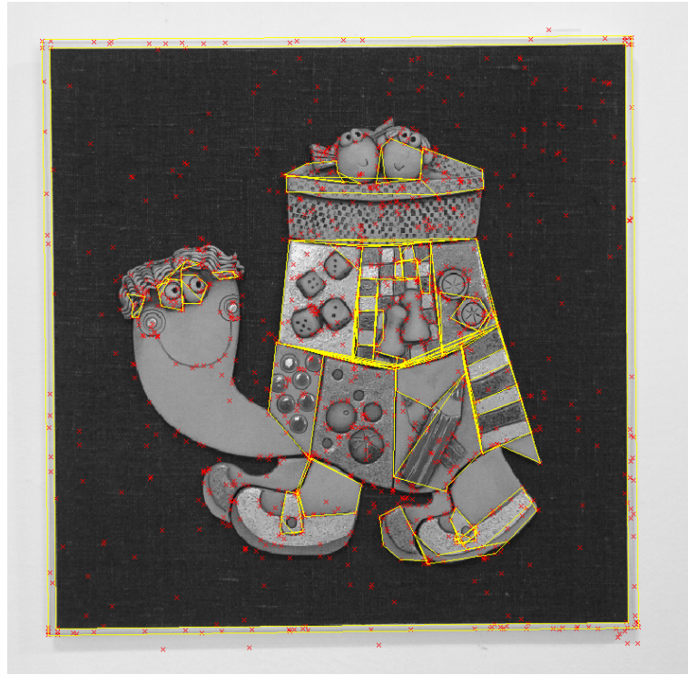
Fig. 1.2: An example of detected polygonal features (yellow) with junctions (red).
