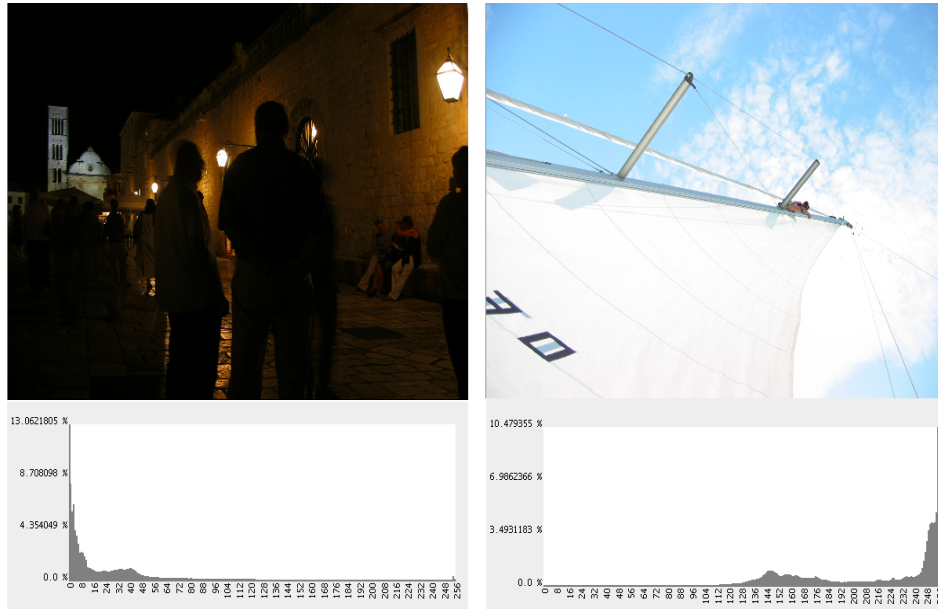
Figure 6.3: Histogram of a dark image (left) and the histogram of a bright image (right).
