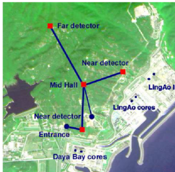
Figure 5: Schematic plan of experimental site. The Daya Bay near detector site is located 363 m from the center of the Daya Bay cores with overburden 98 m of rock (255 m.w.e.). The Ling Ao near detector hall is 481 m from the center of the Ling Ao cores, and 526 m from the center of the Ling Ao II cores where the overburden is 112 m (291 m.w.e). The distances from the far detector to the Daya Bay and to the Ling Ao–Ling Ao II cores are 1985 m and 1615 m, respectively. The overburden is about 350 m (910 m.w.e).
