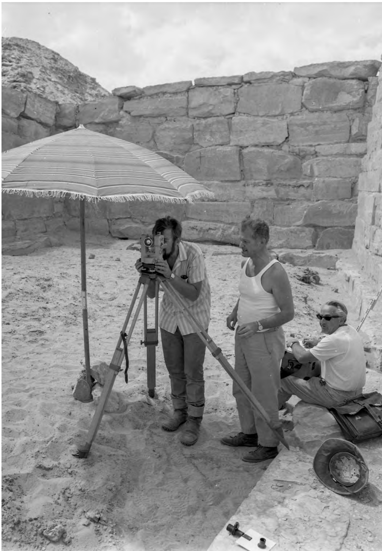
Fig. 3 Geodetic measurement with the theodolite Zeiss Theo 010 in the boat-shaped room of the mastaba of Vizier Ptahshepses (photo M. Zemina)
