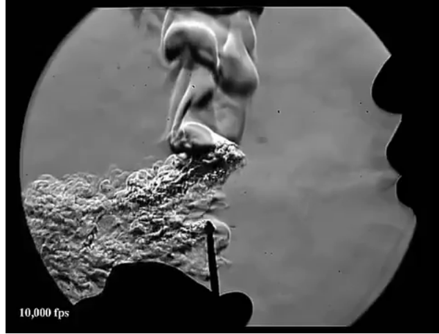
Figure 2.16: Schlieren image of a candle flame. The rich turbulent structure in the left part arose from the breath (from the right side) interacting with the flame. The corresponding video [51] can be seen in the Supplement to this thesis (VIDEO 2)
