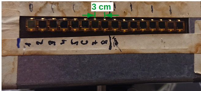
Figure 3.4: The array of photodiodes used to measure the plasma speed above the anode. The photo was taken in 2019
