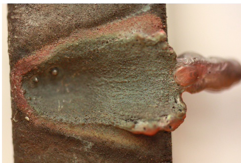
Figure 5.26: Image of the 20 cm wide anode surface after 4 s of operation of the plasma torch when the anode was not rotating. The anode was only cooled down by an internal water circuit. p = 80 kPa, I = 200 A, Ar = 12 slm
