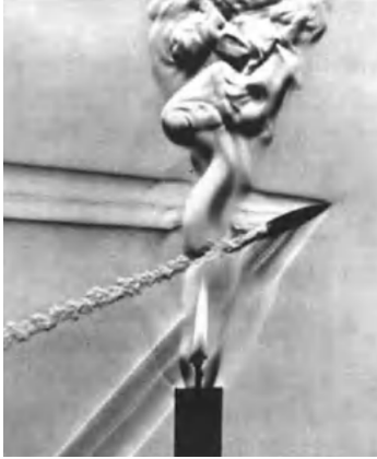
Figure 2.15: Schlieren photo of a bullet and a candle flame [44]
